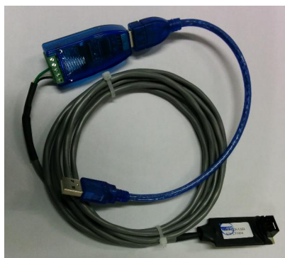
USB/RS-485 Communications Interface with Cable
