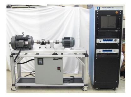
• AC Regenerative Inverters for Motor Test Stands. Example: 400 HP. Customers: Regal-Beloit
